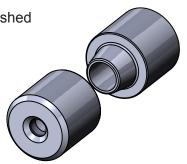
Special Design with Drill & Counterbore for Optional Front/Parting
